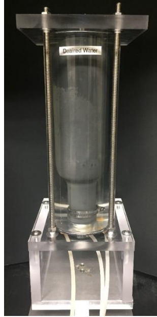
Figure 8: Bladder system supplying water to triaxial test cell volume.
